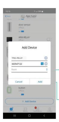
Place the camera of your Smartphone in front of the QR CODE to acquire, automatically, the ID of the relay device
