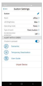
**NOTE**: by activating the PANIC function the ARM-RELAY will remain active leaving the fogging system armed. To restore it, it is needed to manually disarmed it from the App or arm and disarm the alarm system.
